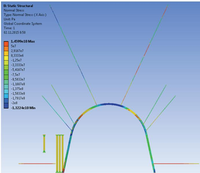
Fig. 5. The curve of horizontal stresses  $\sigma_x$  distribution
