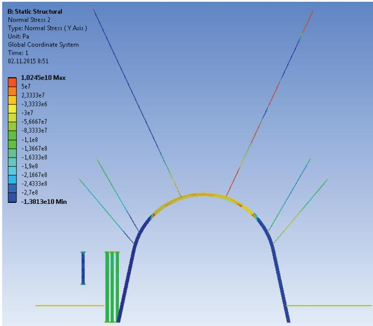
Fig. 4. The curve of vertical stresses  $\sigma_y$  distribution
