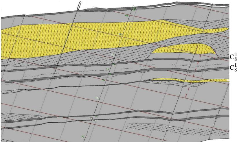
Fig. 1. Fragment of mining and geological section of the area with the most unstable state of the roof rocks in the location of prefabricated drift (scale of 1: 200):
