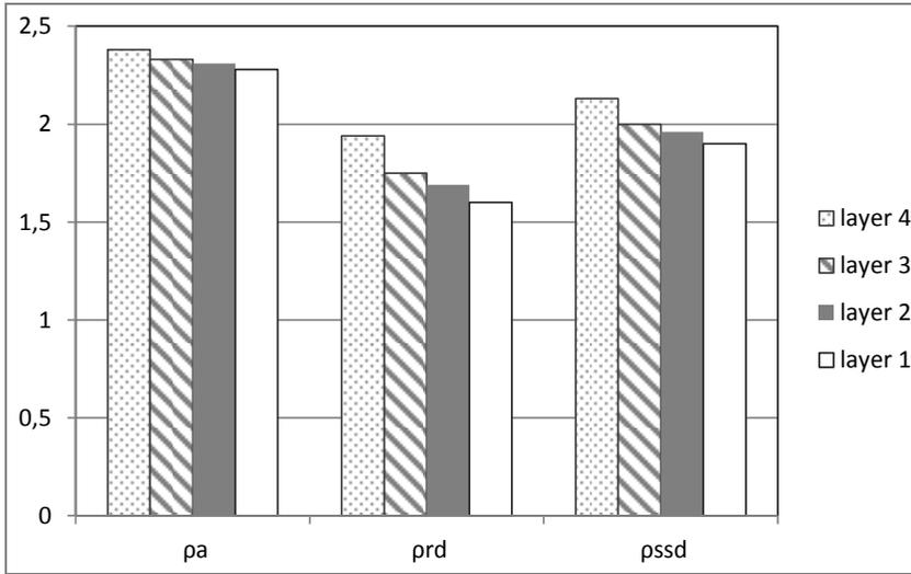
Fig. 5. Density [ $\text{Mg}/\text{m}^3$ ] for chalcidone material 8-16 mm
