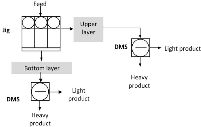
Fig. 8. Scheme of investigations for chalcedonite material 8-31.5 mm
