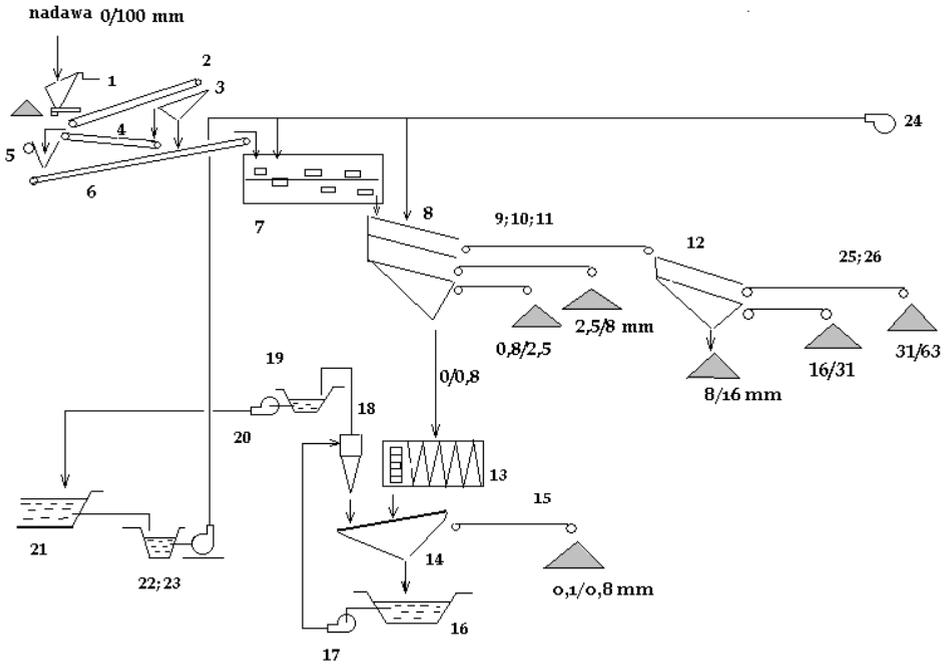
Fig. 1. Technological circuit of chalcidonite processing in "Inowlódz" Mine
