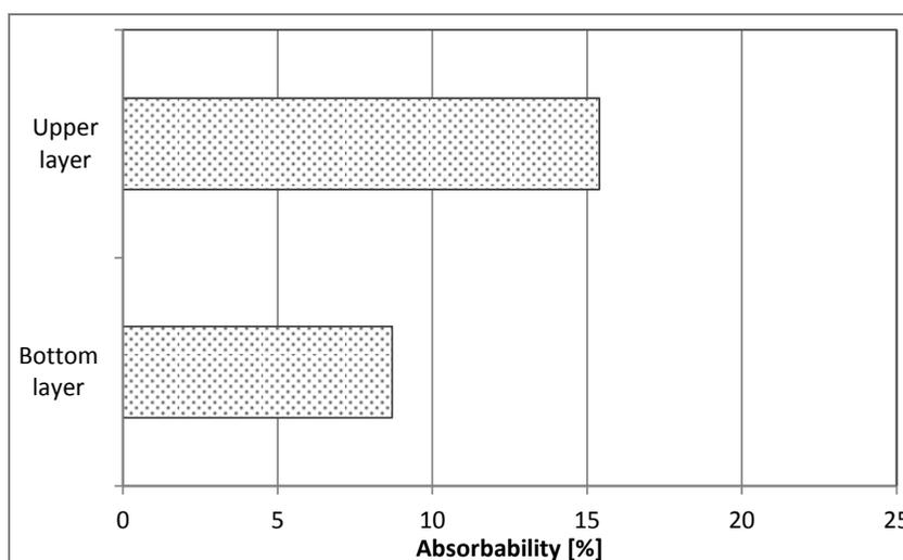
Fig. 7. Water absorption of chalcedonite product 8-31.5 mm
