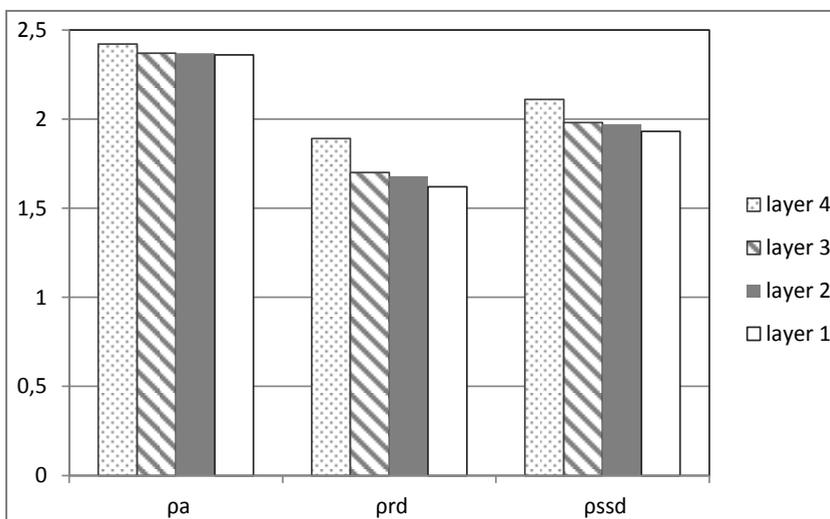
Fig. 4. Density [ $Mg/m^3$ ] for chalcidonite material 4-8 mm
