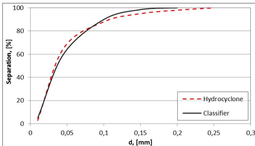
Fig. 2. Separation curves for hydrocyclone and classifier
