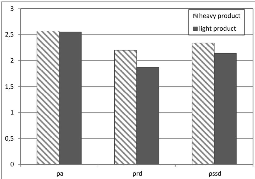
Fig. 9. Density of chalcedonite aggregate separated in DMS with heavy liquid 1.98 [Mg/m<sup>3</sup>]
