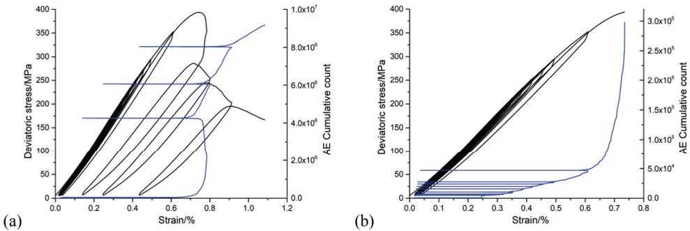
Fig. 8. 20 MPa confining pressure: (a) cumulative count and strain, (b) cumulative count and strain before failure
