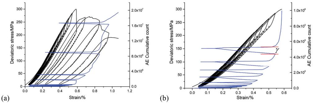
Fig. 7. 10 MPa confining pressure: (a) cumulative count and strain, (b) cumulative count and strain before failure
