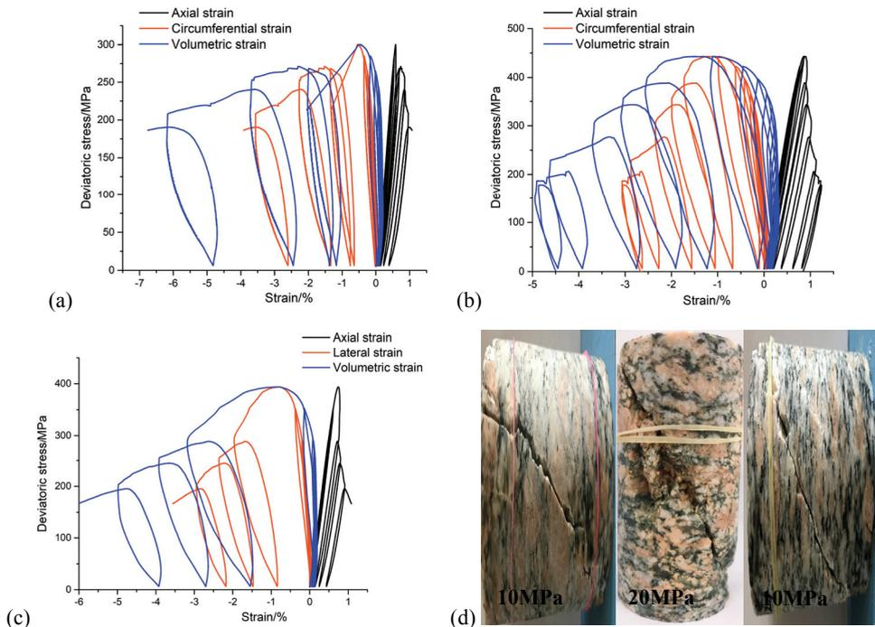
Fig. 5. Confining pressure and failure patterns:
