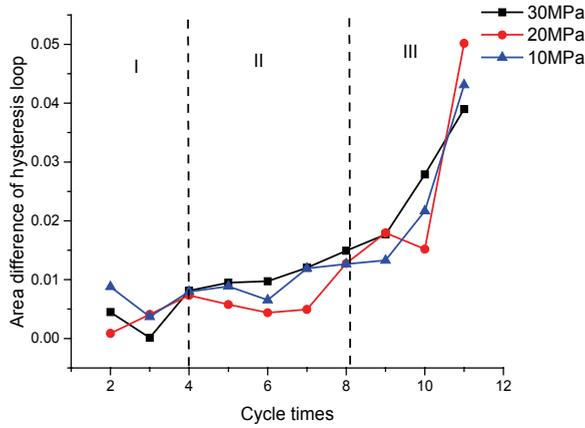
Fig. 10. Area difference of hysteresis loop with cycle times
