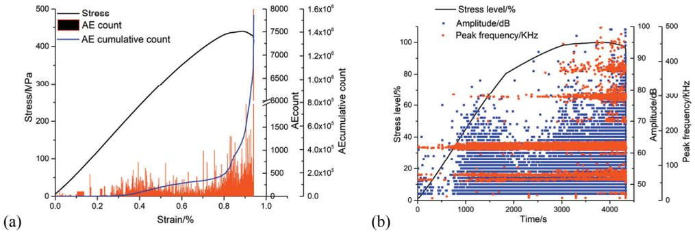
Fig. 4. 30 MPa confining pressure: (a) count and cumulative count, (b) amplitude and peak frequency
