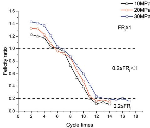
Fig. 11. Felicity ratio with cycle times
