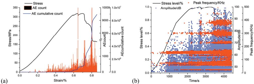
Fig. 2. 10 MPa confining pressure: (a) count and cumulative count, (b) amplitude and peak frequency
