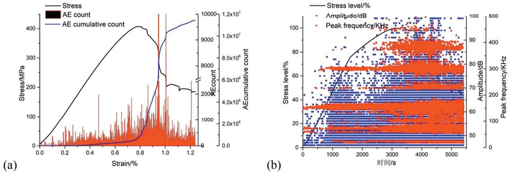
Fig. 3. 20 MPa confining pressure: (a) count and cumulative count, (b) amplitude and peak frequency
