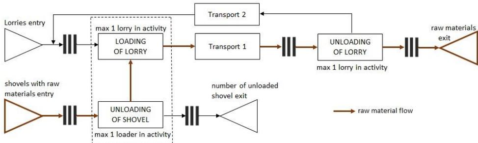
Fig. 1. Technological process at a quarry
