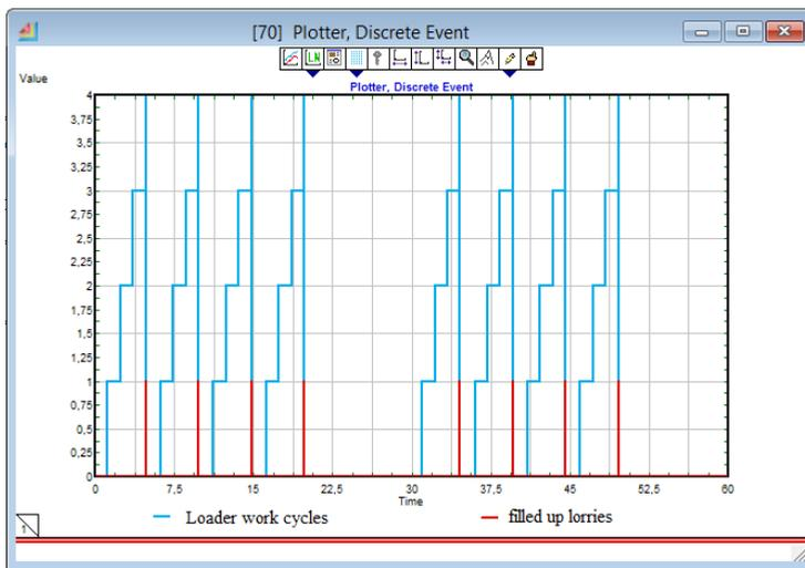
Fig. 3. Loading the lorries by the loader in EXP 1C
