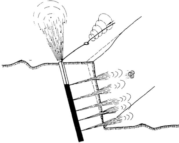
Fig. 1. Air blast fronts in blasting (Jimeno et al. 1995)
