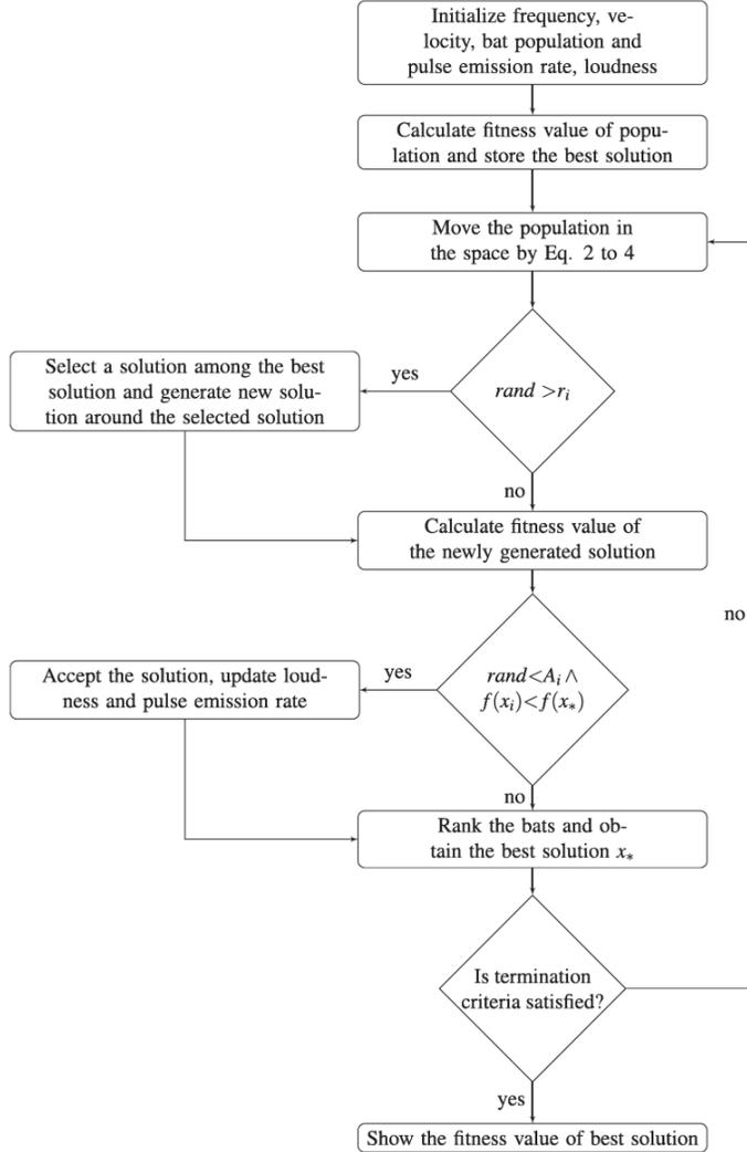
Fig. 2. Flowchart of bat algorithm
