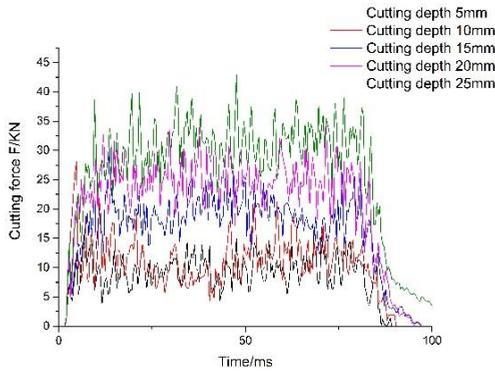
Fig. 8. Cutting force analysis diagram when cutting angle is 40°
