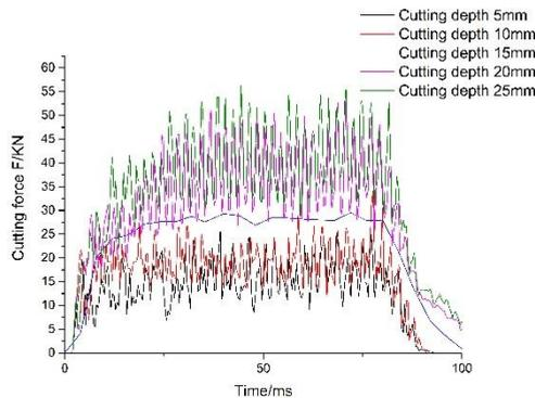
Fig. 6. Cutting force analysis diagram when cutting angle is  $30^\circ$
