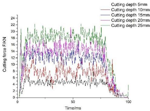
Fig. 9. Cutting force analysis diagram when cutting angle is 45°
