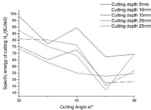
Fig. 15. Analysis diagram of cutting ratio energy consumption
