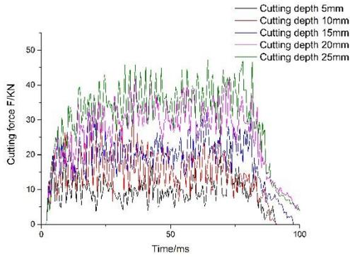
Fig. 7. Cutting force analysis diagram when cutting angle is 35°
