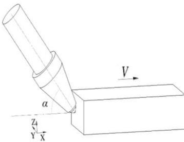
Fig. 3. Diagram of rock cutting by conical pick
