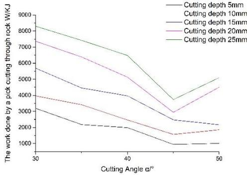
Fig. 14. Diagram of total work of rock cutting by conical pick
