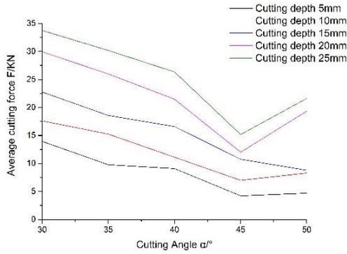
Fig. 11. Average cutting force analysis diagram
