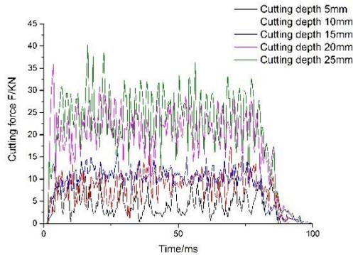
Fig. 10. Cutting force analysis diagram when cutting angle is 50°
