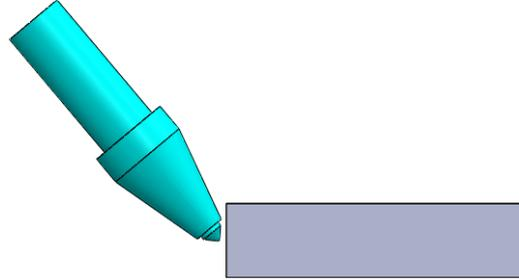
Fig. 2. Diagram of conical pick and rock model
