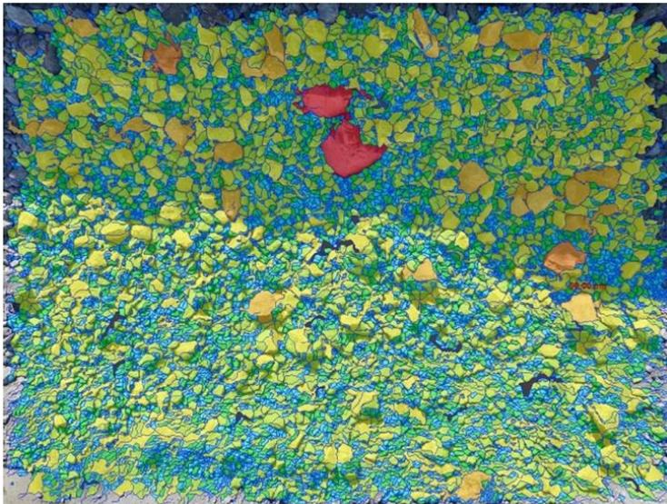
Fig. 4. Color classification of the size of detected grains in the WipFrag program
