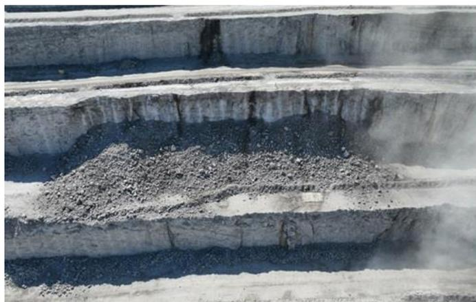
Fig. 1. General view of the muck pile for which a grain size distribution analysis was conducted
