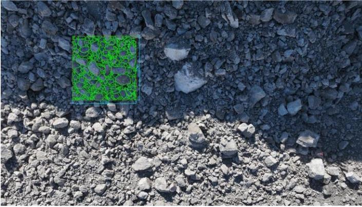
Fig. 2. Selected representative fragment for analysis with digitize boundaries of grains
