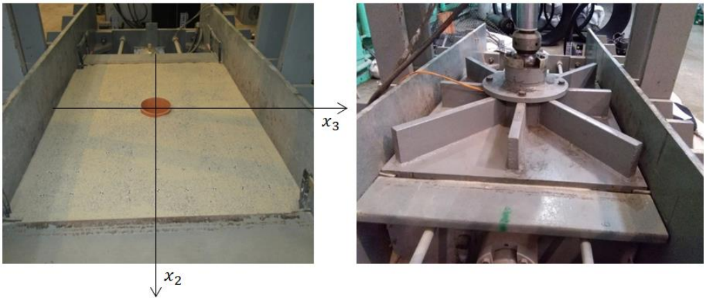
Fig. 3. Test stand box with a model of a flexible manhole riser in the soil (left) and a rigid steel plate which enables simulating vertical load on the soil (right)
