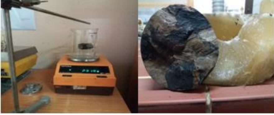
Fig. 8. Determination of volumetric weight with paraffin
