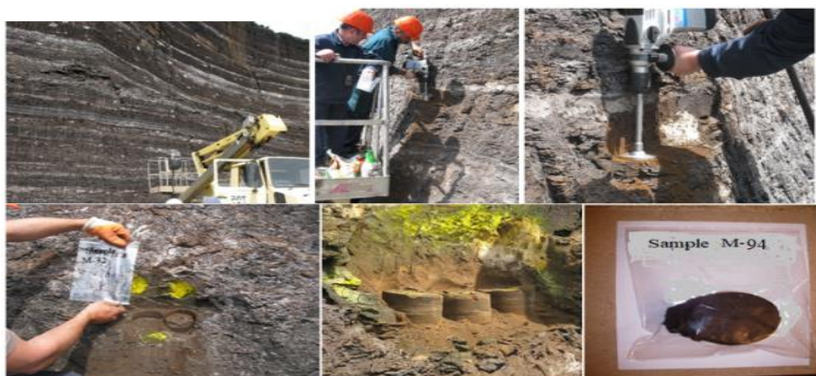
Fig. 4. In-situ sampling procedure on coal cascades
