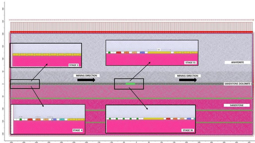
Fig. 4. Numerical model for the remnant width 60 m
