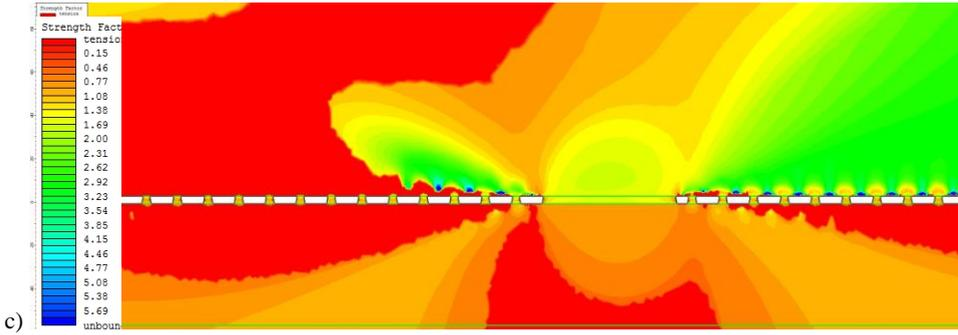
Fig. 6. Distribution of strength factor  $S_f$  for the front distance approximately:
