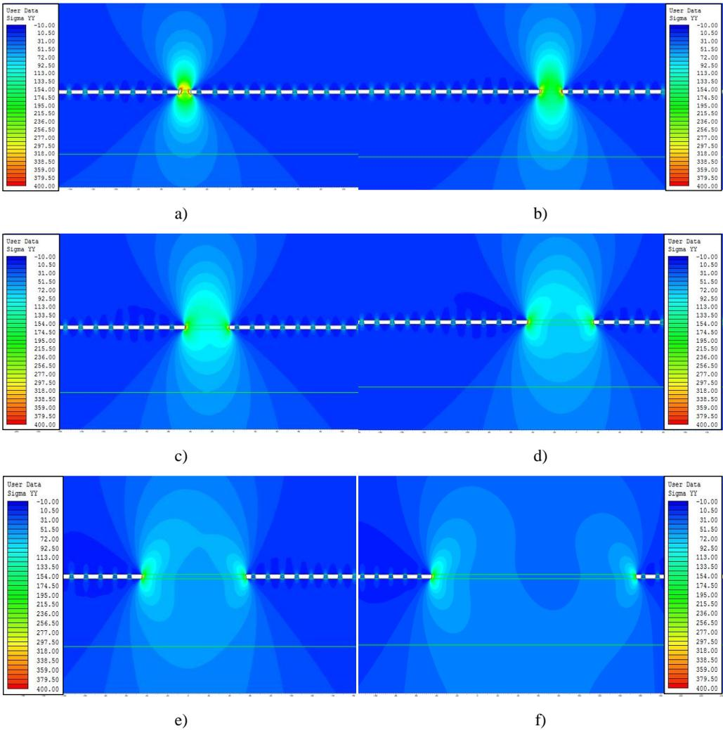
Fig. 5. Distribution of vertical stresses  $\sigma_y$  for the front distance approximately 400 m from the remnant edge – 59th calculation step for different remnant width: a) 10 m, b) 20 m, c) 40 m, d) 60 m, e) 100 m, f) 200 m
