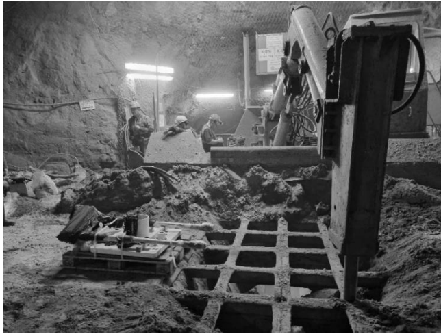
Fig. 2. The unloading point of mined material, popularly called the grate, O/ZG Rudna
