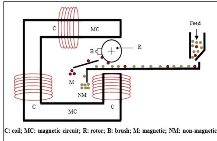
Fig. 1. Magnetic separator high intensity of laboratory (MSHI)
