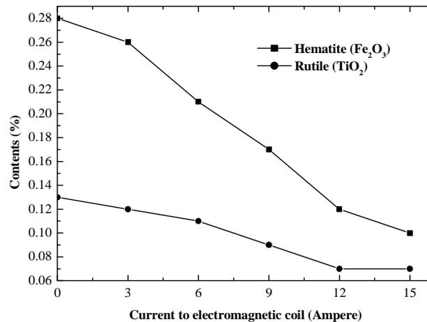
Fig. 4. Effect of current intensity the coil on contents of iron and rutile removal
