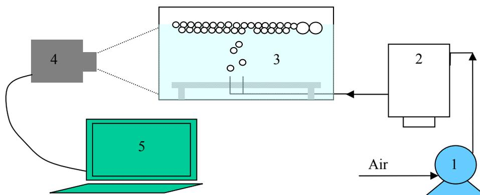
Fig. 4. Experimental set up for CCC measurements:
