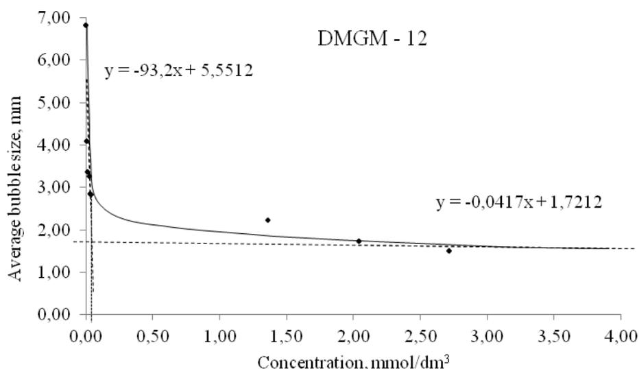
Fig. 5. Critical coalescence concentration (CCC) for DMGM-12
