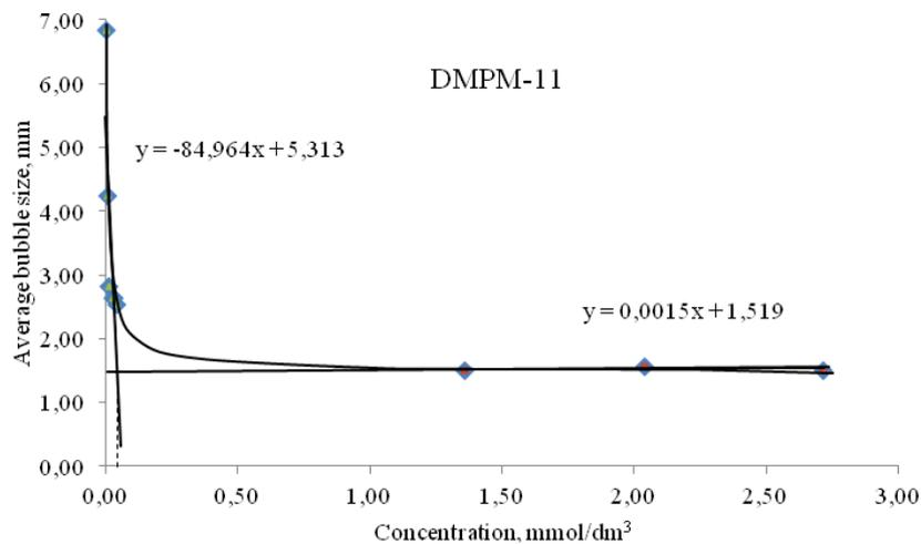
Fig. 9. Critical coalescence concentration (CCC) for DMPM -11
