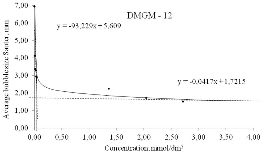
Fig. 6. Critical coalescence concentration (CCC) for DMGM-12
