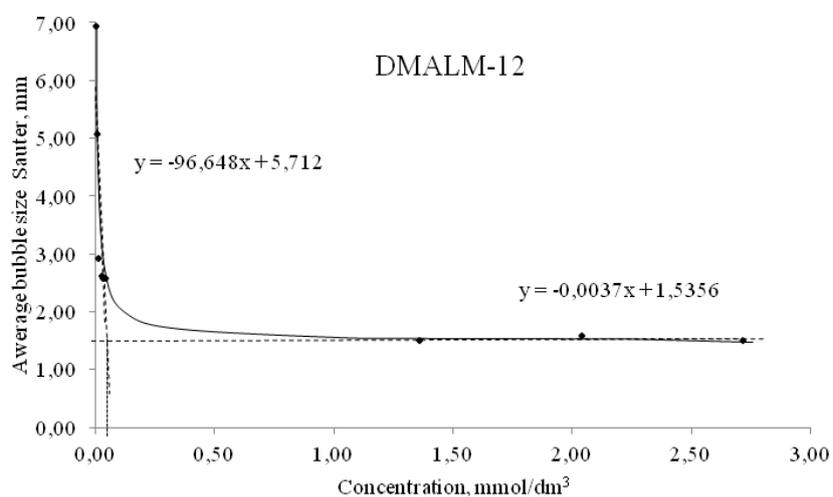
Fig. 8. Critical coalescence concentration (CCC) for DMALM-12
