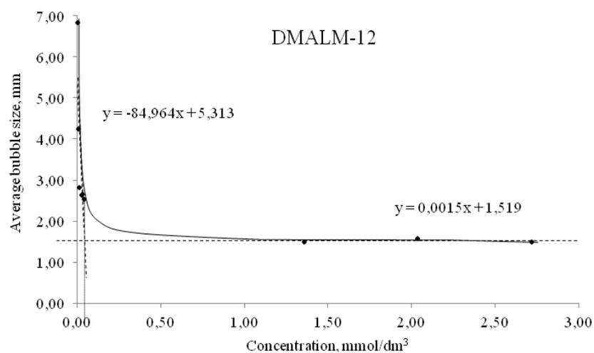
Fig. 7. Critical coalescence concentration (CCC) of DMALM-12
