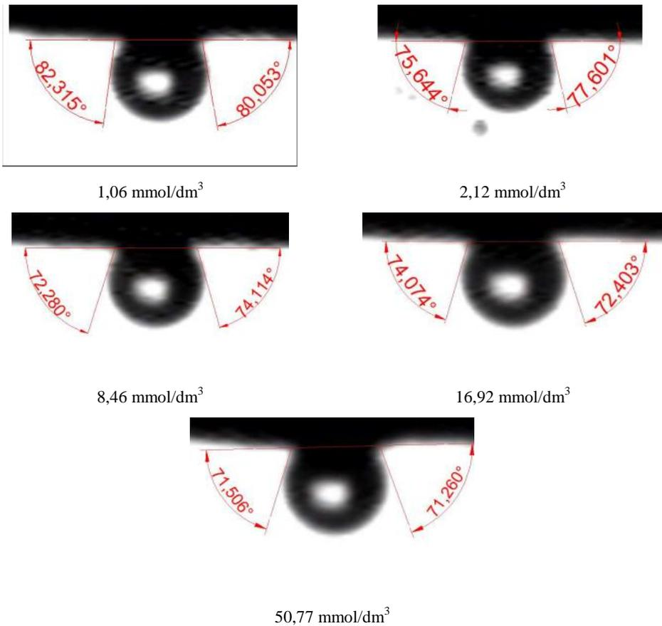
Fig. 3. Measurement of contact angle of copper-bearing shales immersed in aqueous solutions of ethylene glycol butyl ether ( $\text{C}_4\text{E}_1$ ) using captive bubble method (precision of the measurement results as shown by the program)
