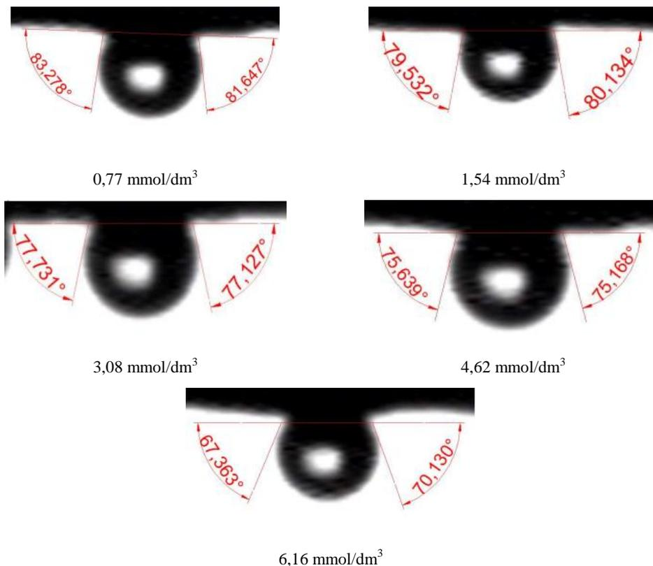
Fig. 4. Measurement of contact angle of copper-bearing shales immersed in aqueous solutions of diethylene glycol butyl ether ( $C_4E_2$ ) using captive bubble method (precision of the measurement results as shown by the program)
