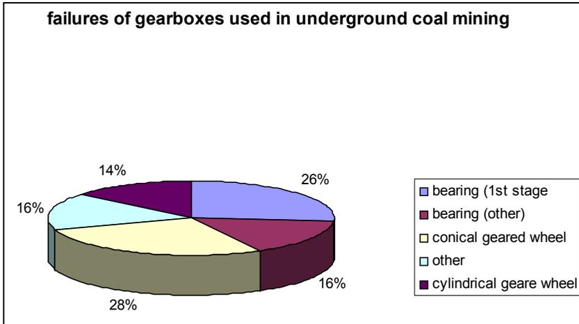
Fig. 10. Percentage of failures for gearboxes used in underground coal mine [6]
