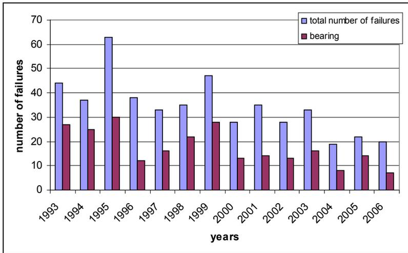
Fig. 14. Failure analysis for pulleys (number of total failures and with respect to bearings)
