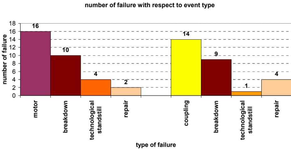
Fig. 21. Number of failures related to DU elements with respect to type of event (gearbox and pulley)
