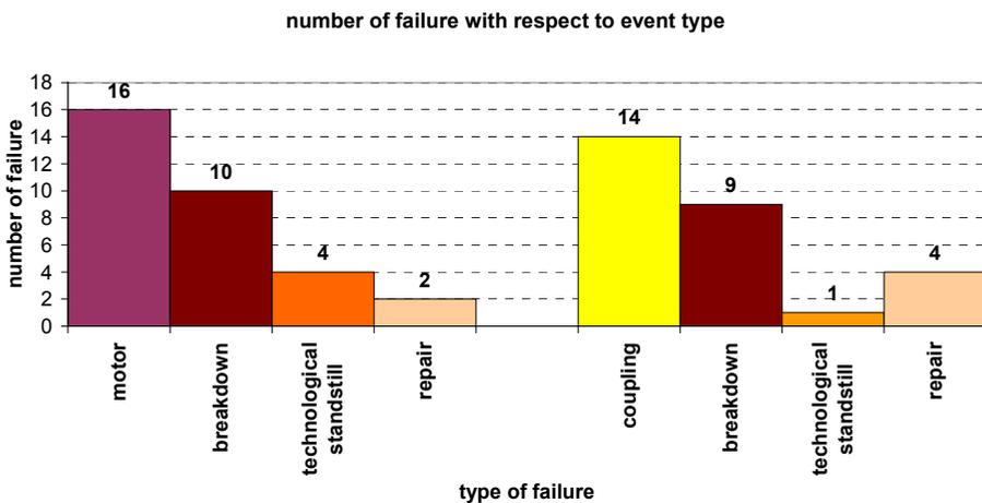
Fig. 20. Number of failures related to DU elements with respect to type of type of event (motor and coupling)
