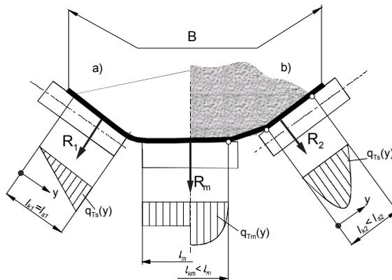
Fig. 22. Distribution of load along belt-idler contact area [9]
