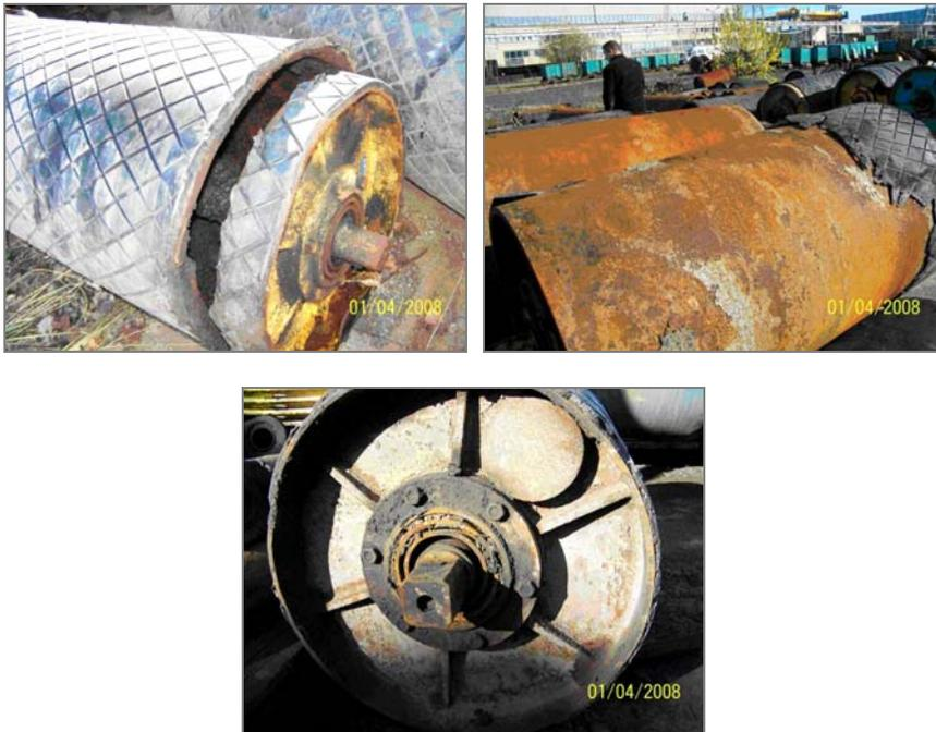
Fig. 15. Examples of pulleys faults (underground mine)
