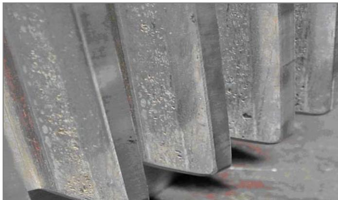
Fig. 11. Example of worn geared wheel
