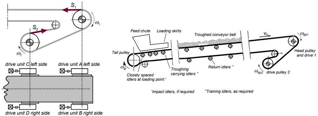
Fig. 3. scheme of belt conveyor [1]
