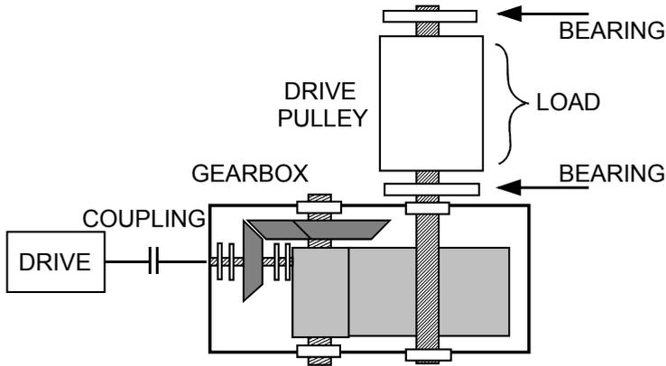
Fig. 8. scheme of drive unit used in CBS
