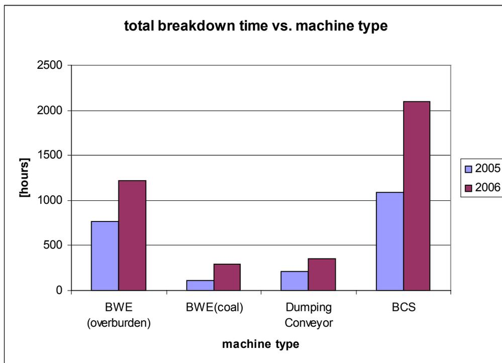
Fig. 7. Comparison of breakdown time for different machines (one mine) [4]
