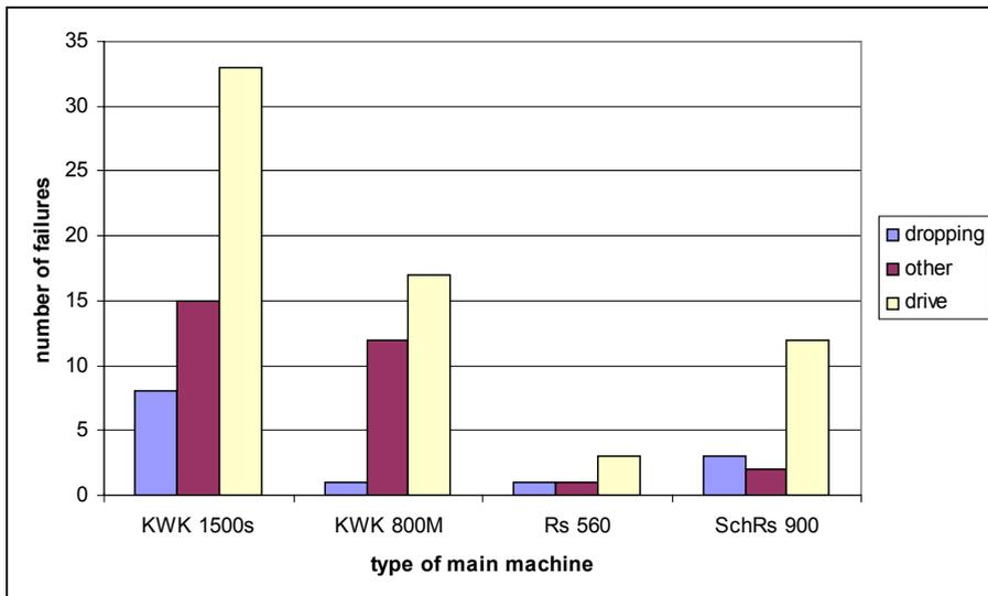
Fig. 13. Number of failures for different types of pulleys used in mine machines in lignite mine
