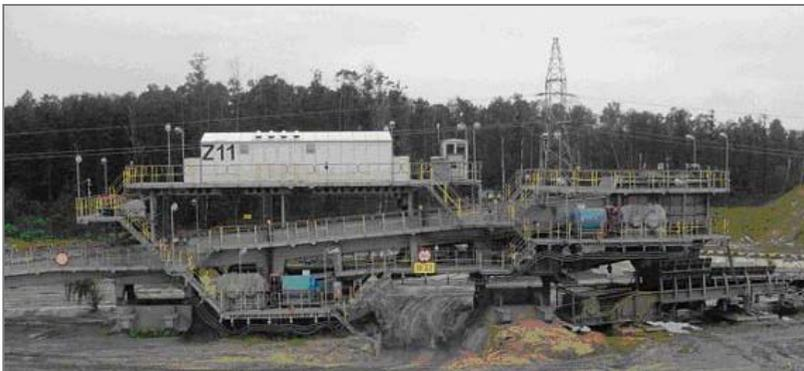
Fig. 4. View on drive units (drive station in (opencast mining))
