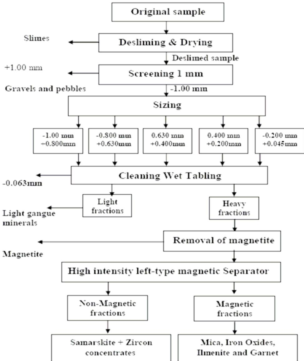
Fig. 9. A proposed flowsheet for beneficiation of samarskite, and zircon from Ras Baroud stream sediments
