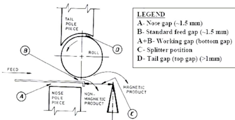
Fig. 8. Gap adjustment diagram for the high intensity lift-type magnetic separator
