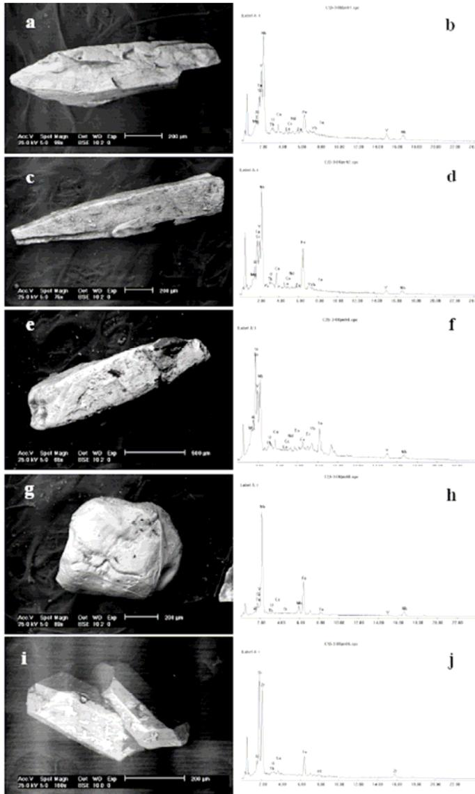
Fig. 3. a-f – backscattered electron image of samarskite and corresponding EDX analyses, g-h – BSE image of columbite grain and its spectrum, i-j – backscattered image of magnetic zircon crystals and their semiquantitative analysis
