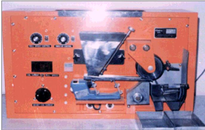
Fig. 7. The high intensity left-type magnetic separator, (Carpc), Model MLH (13) 111–5
