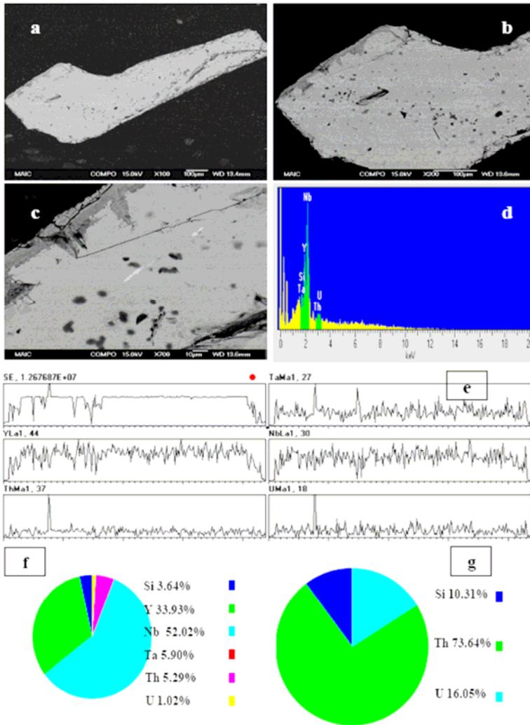
Fig. 4. a–d – backscattered electron images of samarskite crystal showing the bright thorite inclusions and EDX analysis, e – scan line elemental analyses of samarskite, f, g – Elemental composition of samarskite and thorite
