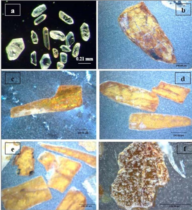
Fig. 2. a) Colorless prismatic zircon crystals, binocular microscope, b) Bloody red samarskite crystal, Crossed Nicolas, c-d) Samarskite crystal of rod-like shape, Polarized light, e) Massive granular samarskite crystals of bright yellow color, Polarized light, f) Massive granular samarskite of dark yellow color, Crossed Nicolas
