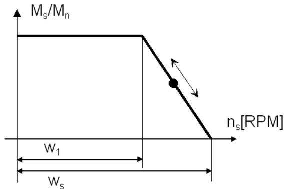
Fig. 11. Electric motor characteristic;  $M$  [Nm],  $W$  [rad/s],  $n_s$  [RPM]
