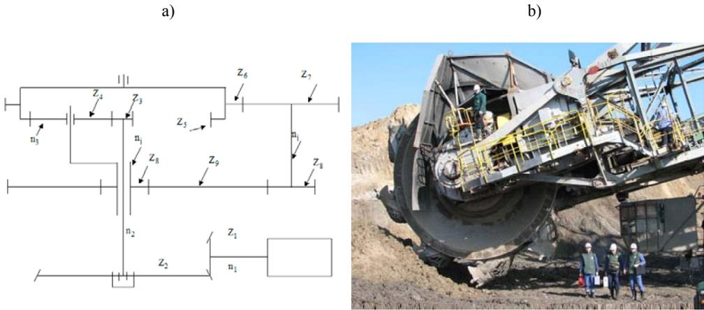
Fig. 4. Diagnosed object: a) scheme of gearbox, b) view of machine
