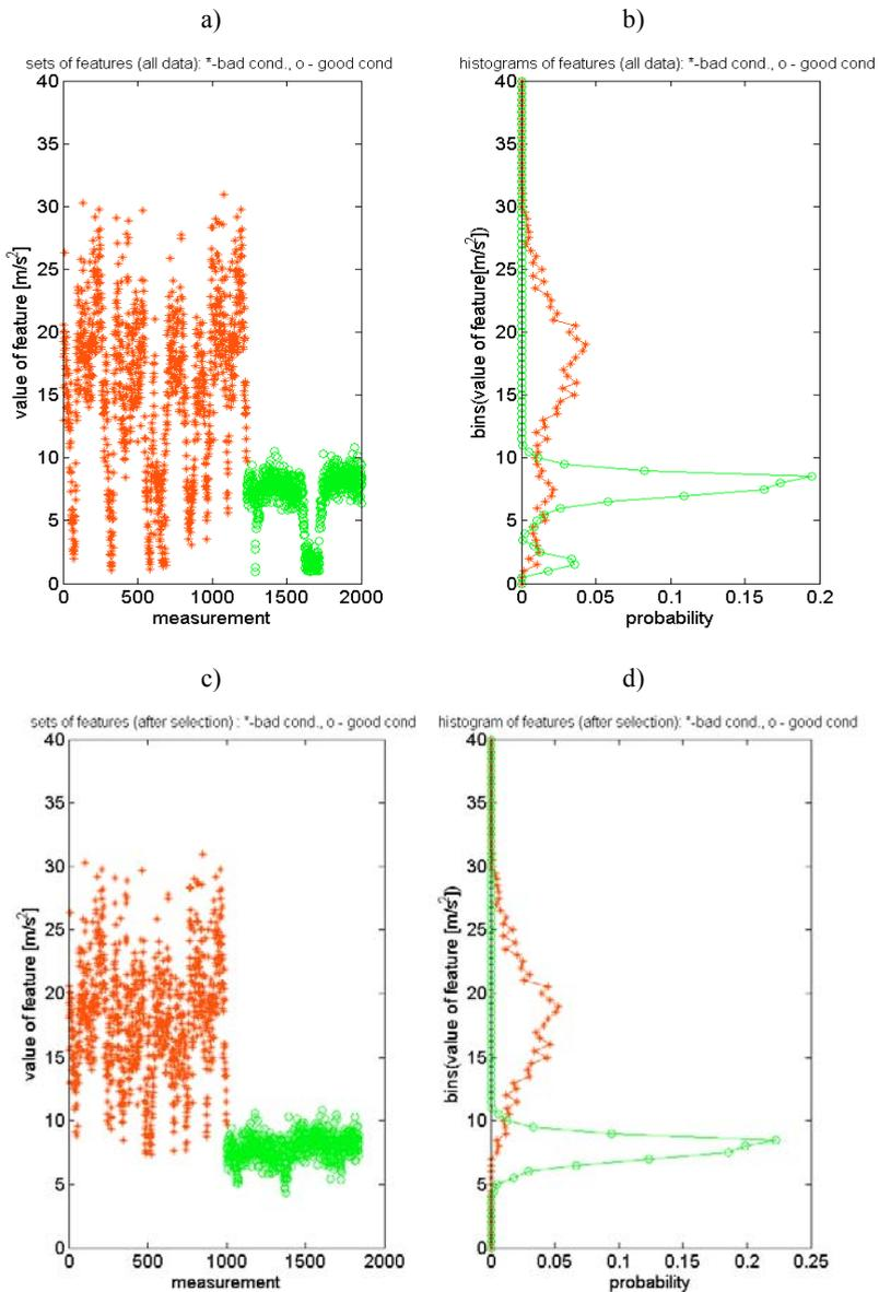
Fig. 6. Probability of feature distributions for two diagnosed objects: circle marked distribution for object in good condition and star marked distribution for object in bad condition; a) for all measurements b) for measurements with properly loaded gearboxes
