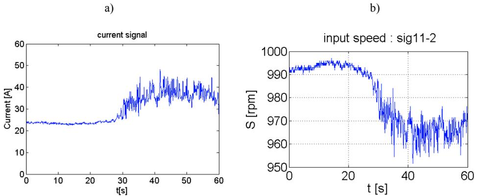
Fig. 2. Values variation as function of time [s]: a) instantaneous electric current consumption in [A], b) instantaneous input shaft rotational speed [RPM]
