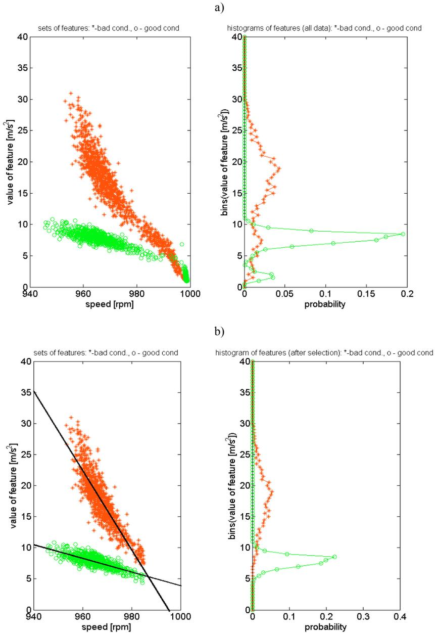
Fig. 10. Distribution of features for bad (stars) and good (circles) condition as function of instantaneous speed and its probability: a) full range of operating speed, b) limited range of operating speed for properly loaded gearboxes (linear relation only)
