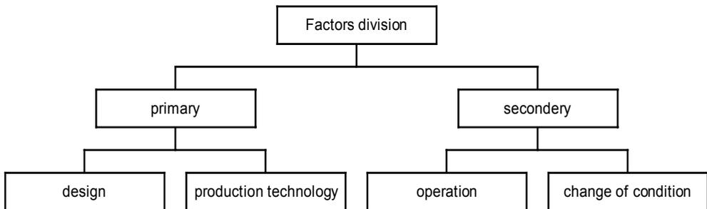
Fig. 3. Introductory division of factors influencing vibration signals
