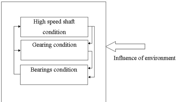
Fig. 6. Interaction of gearbox elements and influence of environment [5]
