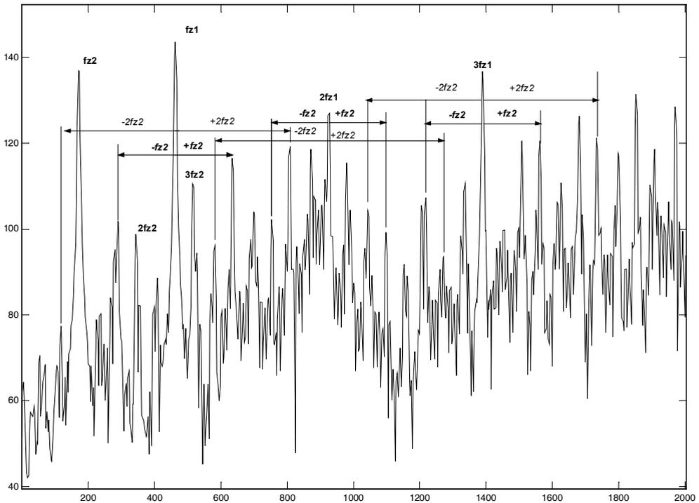
Fig. 1. Vibration spectrum of the signal obtained by computer simulation using the model given in [7]:  $f_{z1}$ ;  $2f_{z1}$ ;  $3f_{z1}$  – meshing frequency and its components for first stage of gearbox and for second stage:  $f_{z2}$ ;  $2f_{z2}$ ;  $3f_{z2}$ ; modulation components:  $-f_{z2}$ ;  $+f_{z2}$  and  $-2f_{z2}$ ;  $+2f_{z2}$  [7]
