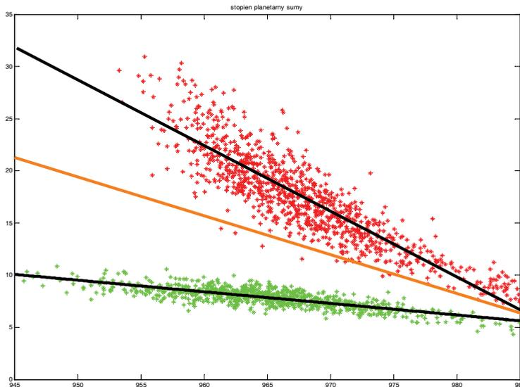
Fig. 4. Statistical regression models for two planetary gearboxes in good and bad condition
