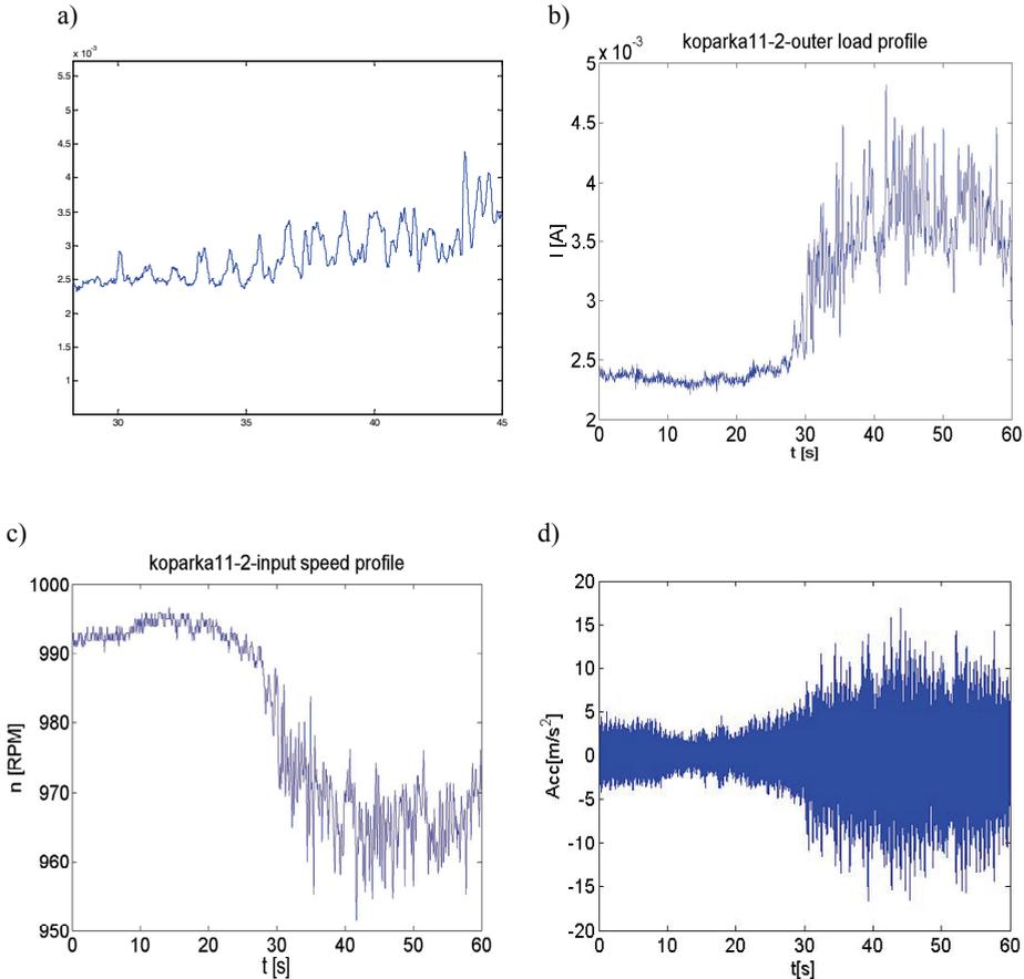
Fig. 2. Variation in: a) general electric current consumption, b) instantaneous electric current consumption, c) input shaft rotation speed RPM, d) vibration signal
