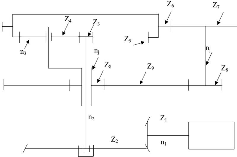
Fig. 5. Bucket wheel driving system
