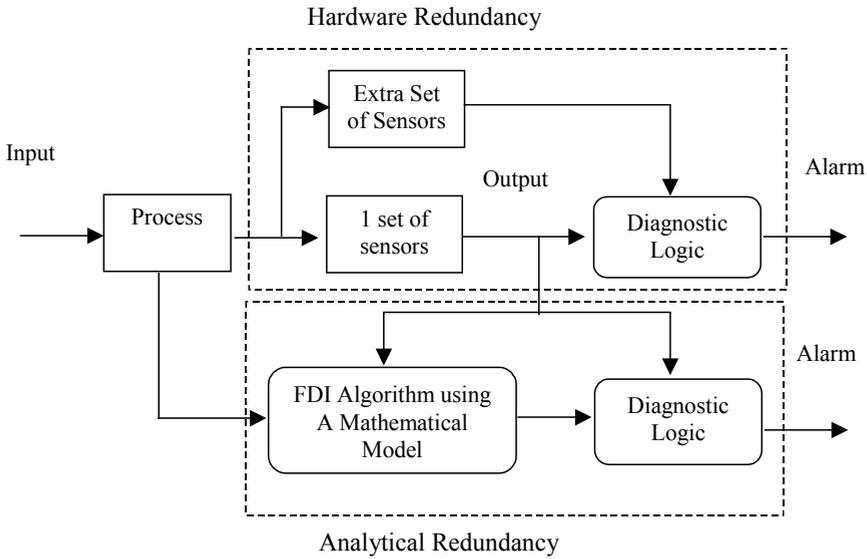
Fig. 3. Hardware vs. analytical redundancy [3]
