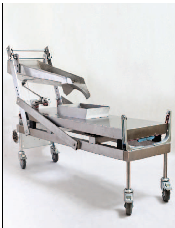
Rys. 4. Analizator AWK B; zakres pomiaru 1–130 mm Fig. 4. AWK B analyser; measuring range 1–130 mm
