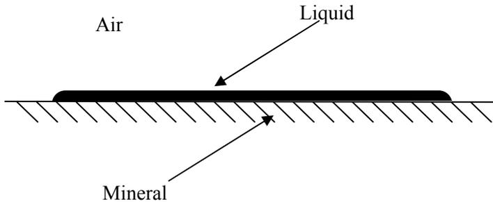
Fig. 2. The drop on the hydrophilic surface
