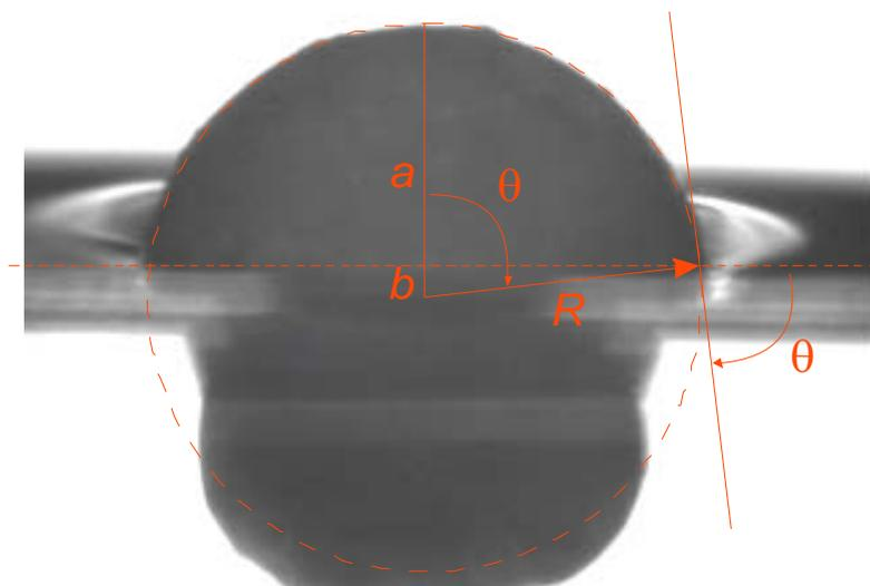
Fig. 4. Dependence of the size of contact angle on the immersion height of the spherical particle of sulfur in water. The liquid surface under the weight of the spherical particle
