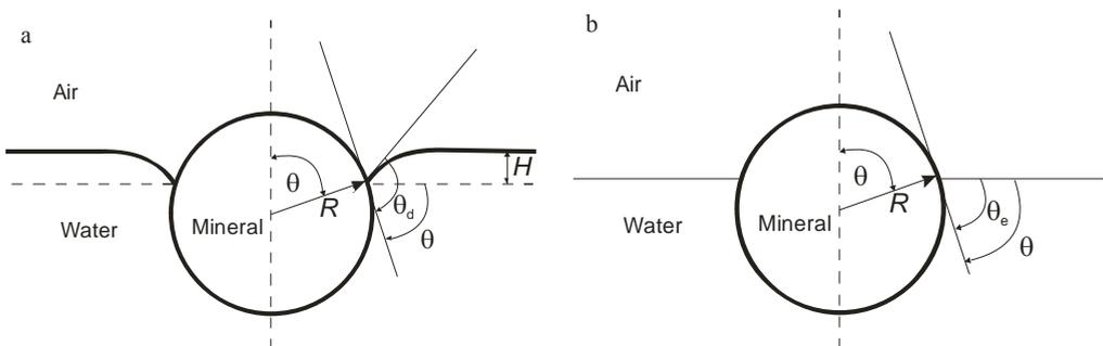
Fig. 14. Spherical hydrophobic mineral particle on the liquid –gas interface: (a) the deflection surface of the water – a concave meniscus (b) a theoretical situation where the line of contact of water with the mineral particle is not deformed (Kowalczyk, Drzymała, 2012)
