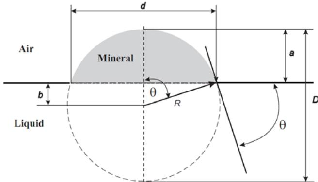
Fig. 13. Spherical solid on liquid surface when the weight of particle is neglected
