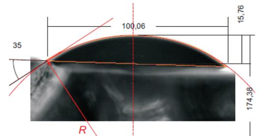
Fig. 11. Water drop on the surface of carbon
