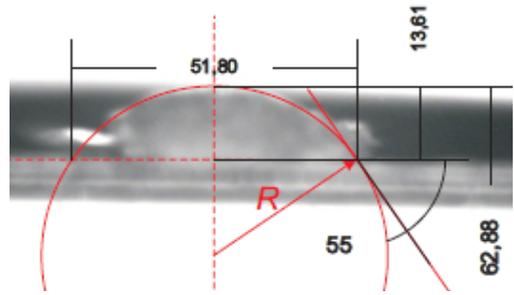
Fig. 16. Spherical particle of color fluorite on water surface
