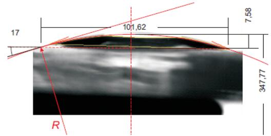
Fig. 9 Water drop on the surface of gypsum
