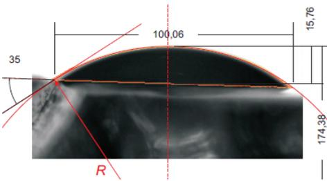
Fig. 10. Water drop on quartz surface
