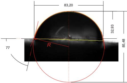
Fig. 6. Water drop on the surface of white fluorite
