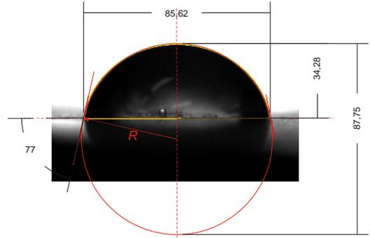
Fig. 7. Water drop on the surface of color fluorite
