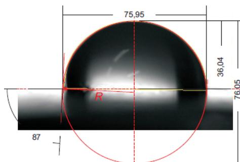
Fig. 12. Water drop on the surface of sulfur
