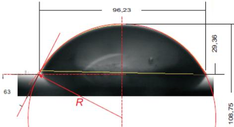
Fig. 8. Water drop on the surface of green fluorite
