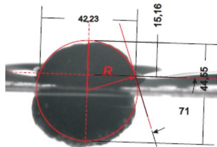
Fig. 20. Spherical particle of carbon on water surface
