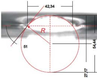
Fig. 15. Spherical particle of white fluorite on water surface
