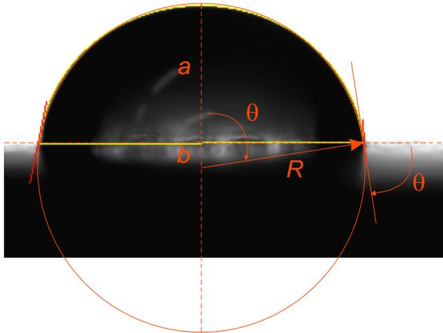
Fig. 3. The drop of water placed on the carbon surface
