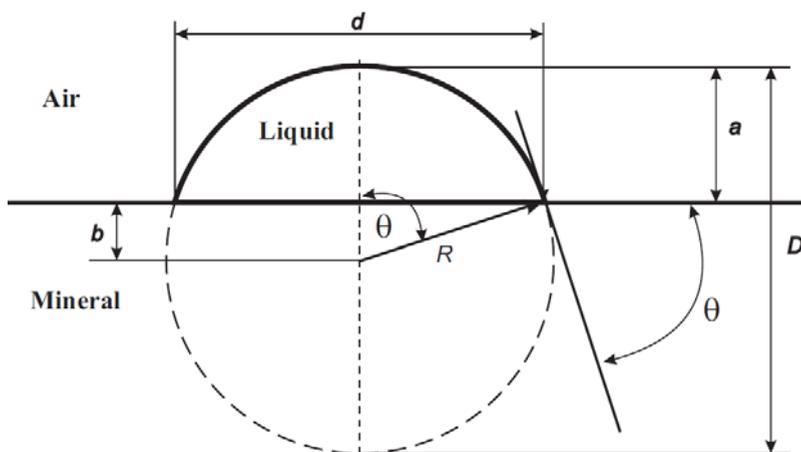
Fig. 5. The graphical representation contact angle measurements for sessile drop
