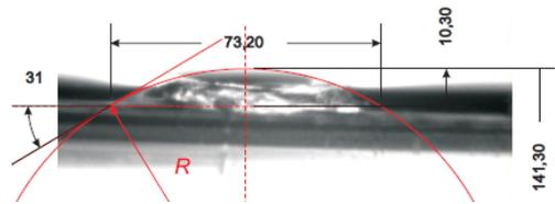
Fig. 18. Spherical quartz particle on water surface
