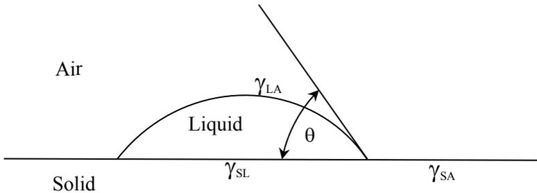
Fig. 1. The drop on a hydrophobic surface, with the graphical presentation of the Young equation
