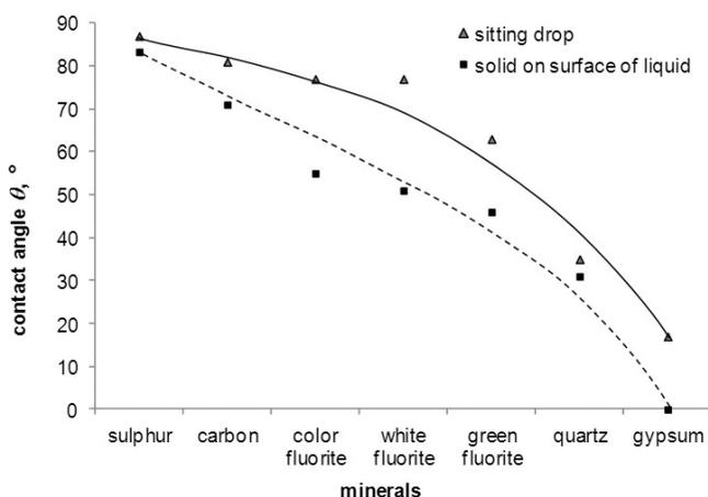
Fig. 23. Contact angle for different materials for sessile drop and solid on the liquid surface
