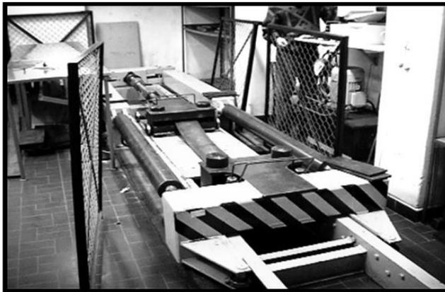
Fig. 1. ZP-40 tensile tester for belt joints (<http://www.ltt.pwr.wroc.pl>)
