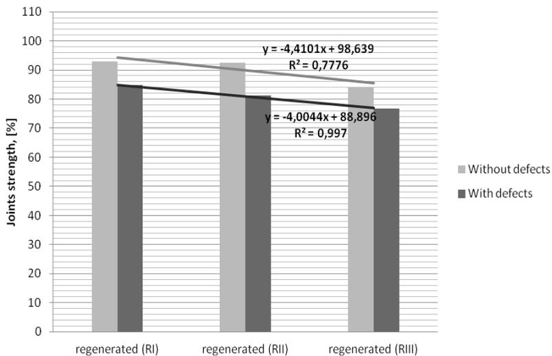
Fig. 7. Average joint strengths in regenerated belts (RI+RII+RIII)
