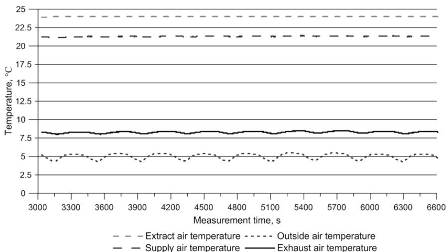
Fig. 2. Sequence of changes in temperature after stabilization system for the outside air temperature of 5°C and 24°C – temperature of removed air
