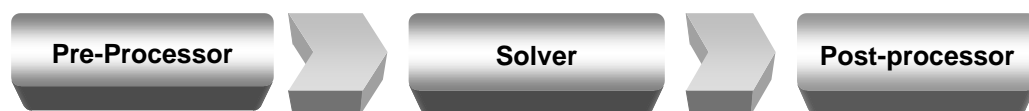
Fig. 2. ANSYS CFX modules: CFX Pre-Processor software – modification in geometry, determination of initial conditions, grid generation; CFX Solver - calculations using multigrid technology for solving equations; CFX Post-Processor – presentation of analysis results, possibility to present different variants of solving equations (Doległo, at al., 2009)
