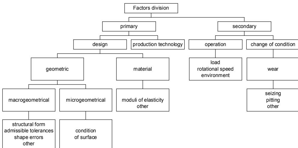
Fig. 6. Factors affecting diagnostic signal or vibro-acoustic effect
