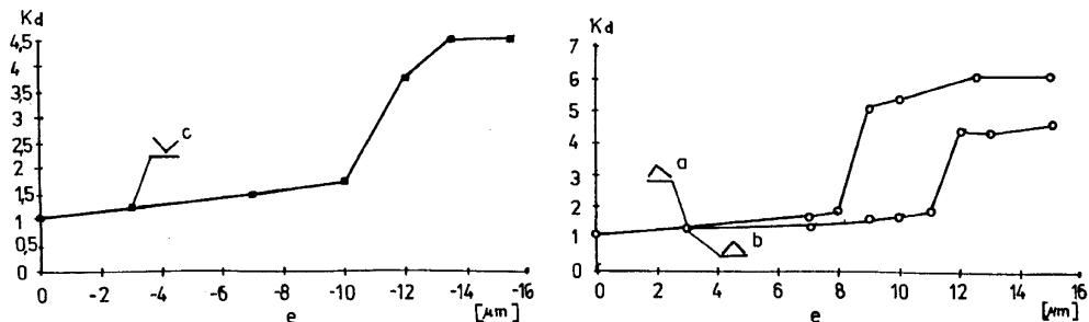
Fig. 7. Coefficient  $K_d$  as function of inter-tooth error and error mode: a –  $E(0.1, e, 0)$ , b –  $E(0.5, e, 0)$ , c –  $E(0.5, -e, 0)$ , according to [1].
