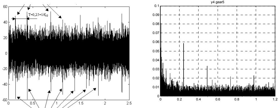
Fig. 10. Acceleration [ $\text{m/s}^2$ ] signal time [s] trace with series of peaks (peaks marked with arrows) and cepstrum for signal
