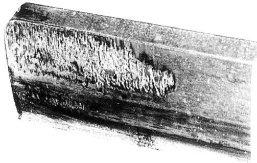
Fig. 2. Image of surface damaged by gear tooth scuffing/seizing (resulting from out-of-parallel meshing of teeth) [3]
