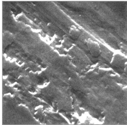
Fig. 3. Electron microscope image of surface damaged by scuffing/seizing (in its initial stage), magnification of 1000x [4]
