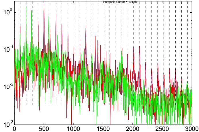
Fig. 13. Spectrum comparing for good (green) and bad (red) object condition
