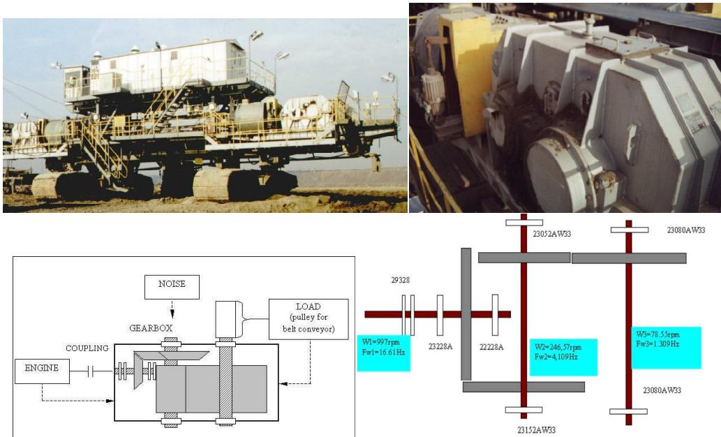
Fig. 1. Belt conveyor driving system
