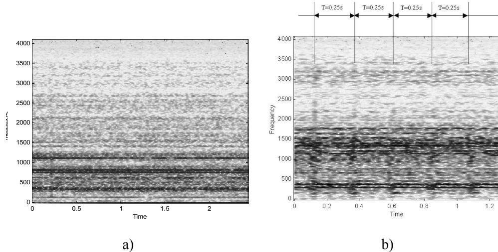
Fig. 11. Time-frequency [s]–[Hz] spectrograms a) spectrogram of signal without regular peaks b) spectrogram of signal with marks equivalent regular peaks.
