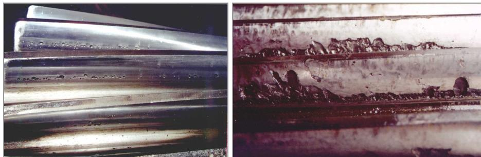
Fig. 4. Pitting and flaking on gear flanks
