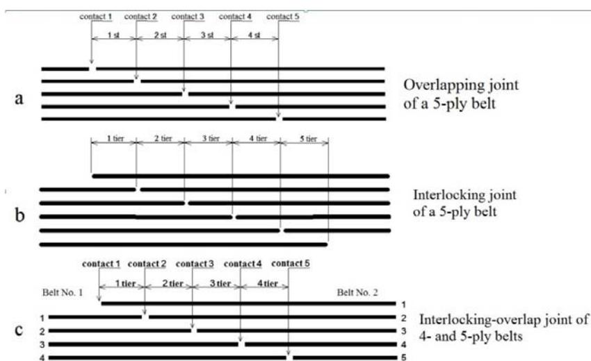
Fig. 1. Typical construction diagrams for multi-ply belts
