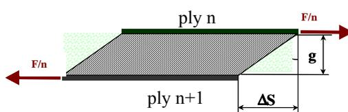
Fig. 4. Adhesive joint deformation diagram
