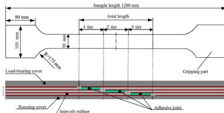
Fig. 3. The shape of a belt joint sample for determining deformations in an adhesive joint
