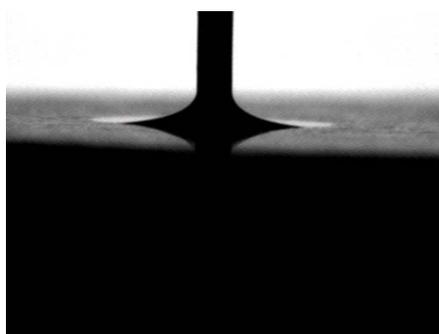
Fig. 3. Example of receding contact angle measurement
