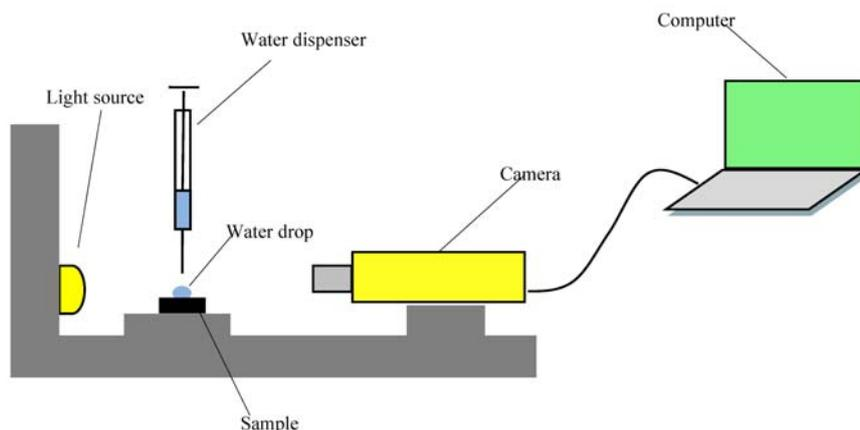
Fig. 4. Scheme system to measurement of contact angle
