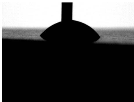
Fig. 2. Example of advancing contact angle measurement
