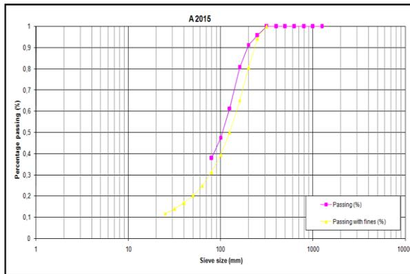
Fig. 8. Fragment size distribution for blast (A 2015)
