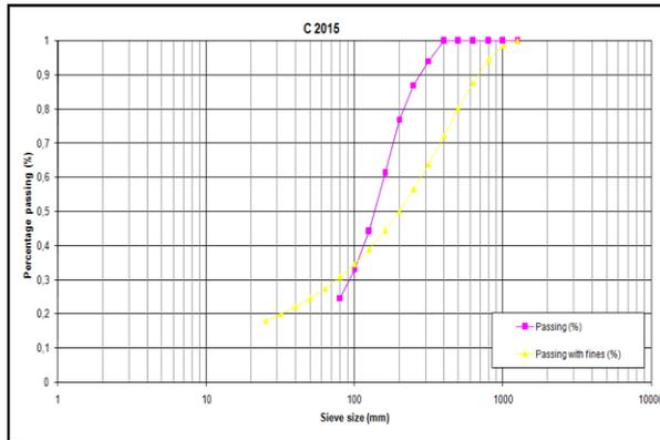
Fig. 10. Fragment size distribution for blast (C 2015).
