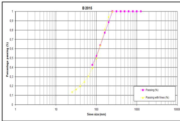
Fig. 9. Fragment size distribution for blast (B 2015).
