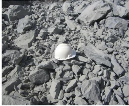
Fig. 7. Visual result of the fragmentation (Amesmesa Blast A 2015)
