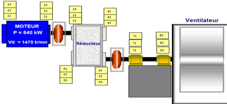
Fig. 5. Block diagram of the fan dispositive
