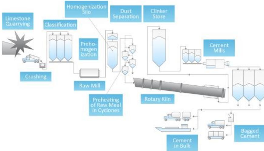
Fig .2 . The cement manufacturing process (www.westchinacement.com)
