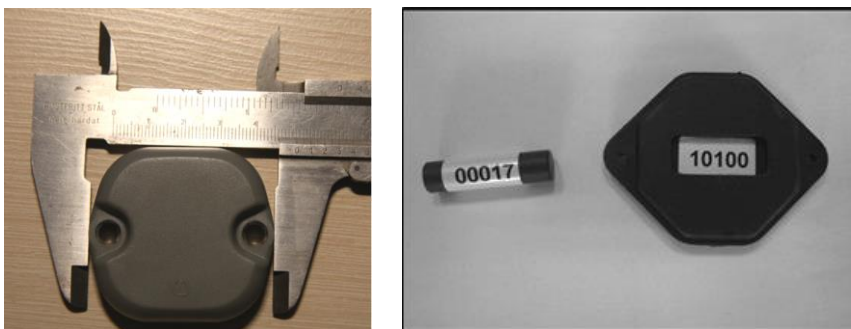
Fig. 2. E-pellets prepared for the experiment: left: Equipment 1, right: Equipment 2 – pellets from Electrotech: “small”, tubular (length 40 mm, diameter: 10 mm) and “big”, hexagonal (length: 75 mm, width: 55 mm, thickness: 10 mm); labels on tags are their written ID
