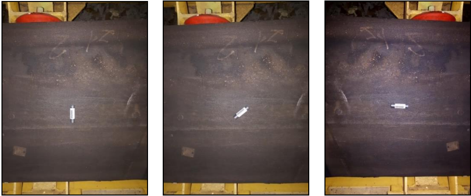
Fig. 4. Possible tubular (A) tags vertical position relative to belt: across, skew, along (left to right, respectively)
