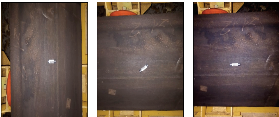
Fig. 4. Possible tubular (A) tags vertical position relative to belt: across, skew, along (left to right, respectively)
