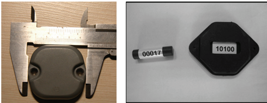
Fig. 2. E-pellets prepared for the experiment: left: Equipment 1, right: Equipment 2 – pellets from Electrotech: “small”, tubular (length 40 mm, diameter: 10 mm) and “big”, hexagonal (length: 75 mm, width: 55 mm, thickness: 10 mm); labels on tags are their written ID (for easier checking the test results)
