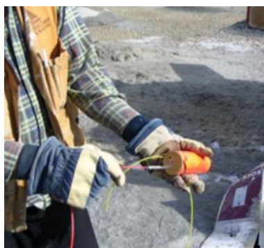
Fig. 5. Operator performing priming tasks with a booster and a Nonel detonator, emphasizing the importance of technical training to ensure safe and efficient procedures
