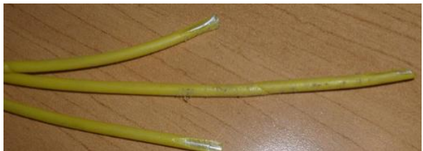
Fig. 11. Remnants of transmission tube that failed to initiate during the blast, highlighting a disruption in the detonation sequence
