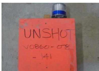
Fig. 2. Warning sign and beacon used to mark an uninitiated borehole, ensuring safety measures during the handling of undetonated explosives
