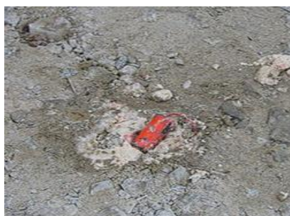
Fig. 1. Detail of a partially exposed booster following a misfire in a blast, associated with operational failures such as errors in layout or delay timing programming
