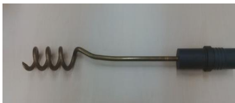
Fig. 8. Flexible tool designed for retrieving cartridges from boreholes. Manufactured from non-sparking materials, such as brass, to ensure safe handling and prevent spark generation
