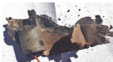
Fig. 13. Remnants of a booster retaining its detonator, indicative of inadequate initiation likely caused by moisture-induced instability
