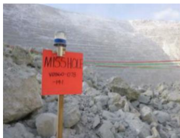
Fig. 7. Example of demarcation and marking of a zone with an undetonated borehole, using visual signals such as warning tapes and flashing lights to ensure safety in the area
