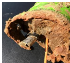
Fig. 14. Detailed view of booster remnants and a NONEL detonator that did not initiate, evidencing incomplete initiation under adverse environmental conditions
