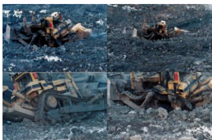
Fig. 3. Bulldozer destroyed after encountering a misfire during ripping, highlighting the hazard of uncontrolled detonations to heavy equipment and operator safety
