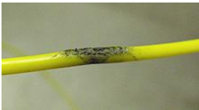
Fig. 10. Transmission tube with an initiation point caused by an incorrect connection, which prevented the tube from activating and resulted in a misfire
