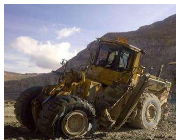
Fig. 4. Front-end loader severely damaged while excavating a booster from an unmarked misfire, underscoring the need for proper marking and strict inspection protocols
