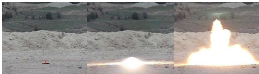
Fig. 9. Sequence of controlled destruction of extracted explosives. The images illustrate the initial ignition, detonation propagation, and energy release in a secure location, adhering to strict safety protocols under expert supervision
